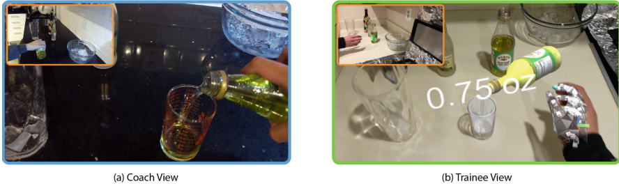
Fig. 1. An illustration of HoloCook. Two individuals, one as a coach and the other as a trainee, each equipped with HoloLens 2, are situated in separate kitchens. As the system starts, the coach’s actions are live-streamed to the trainee’s end. The trainee observes and replicates the actions to complete tasks. (a) and (b) depict the coach’s and the trainee’s perspectives, with side camera views indicated by the top-left orange boxes. In this cocktail-making instance, the coach pours lime juice (0.75 oz) into a measuring cup. Simultaneously, the trainee sees an overlay of the lime juice, the measuring cup, and 3D texts indicating the amount. The trainee follows suit accordingly.
