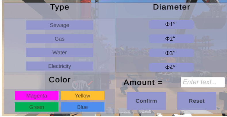
Figure B7 The Drone UI for ordering pipes: This interface appears after the Fetcher presses the AI Drone menu button (Figure B6(b)). After specifying the pipe type, color, diameter, and quantity, the drone (Figure 7(a)) will deliver the requested pipes.
